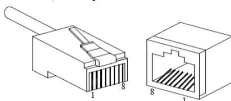
RJ 45 port support automatic MDI/MDI-X operation. can connect the PC , Server, Converter and HUB by straight-through cable wiring . Pin 1, 2, 3, 6 Corresponding connection in MDI. 1→3, 2→6, 3→1, 6→2 are used as cross wiring in the MDI-X port of Converter and HUB. 10Base-T are used in MDI/MDI-X, the define of Pin in the table as below.
